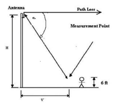
Please note that calculations were performed using the techniques and procedures outlined in the FCC OET Bulletin No. 65 with particular emphasis on the pattern of antennas and the number of channels per sector.
